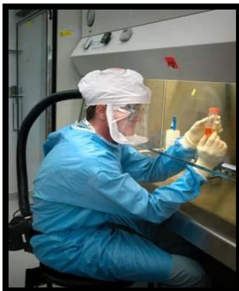
Figure A-3. Class II BSCs do not provide total barrier containment.
