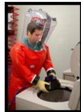
Figure 1-7. Researcher in BSL-4 PPE placing a rotor in a centrifuge.
