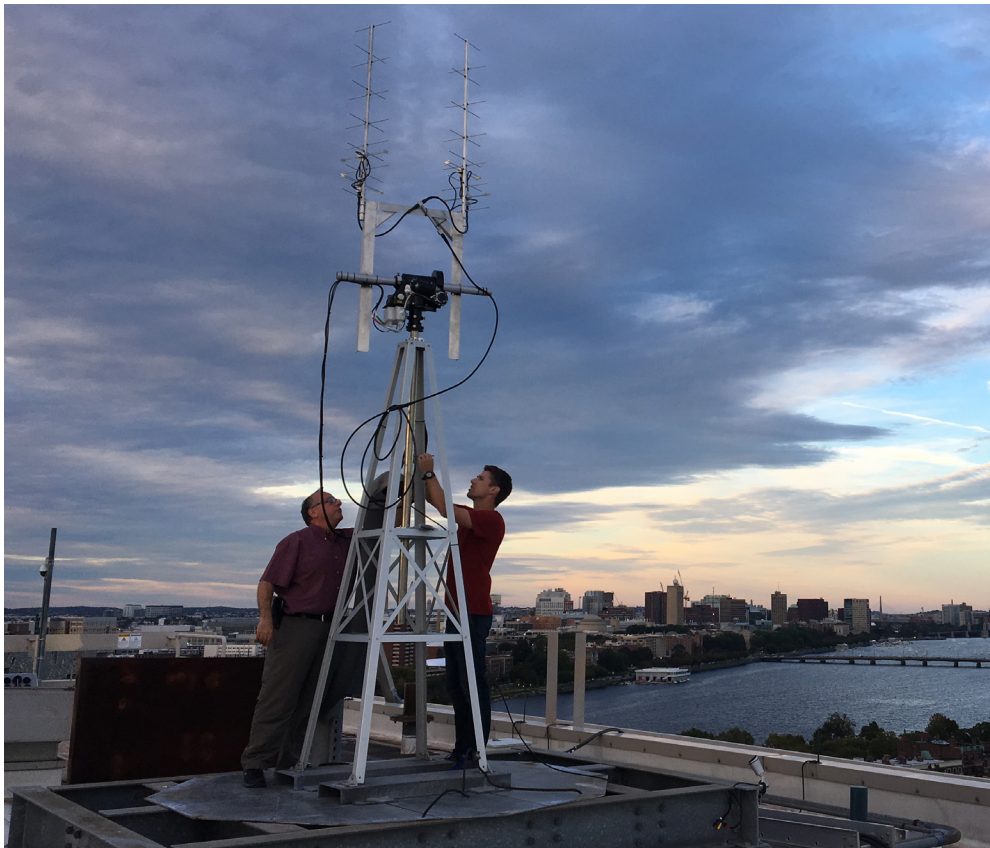
The CuPID Cubesat Observatory team puts the finishing touches on the ground station on the roof of Photonics. The antenna will be used for radio communication with the spacecraft in orbit. (Photo Courtesy of Assistant Professor Brian Walsh)
