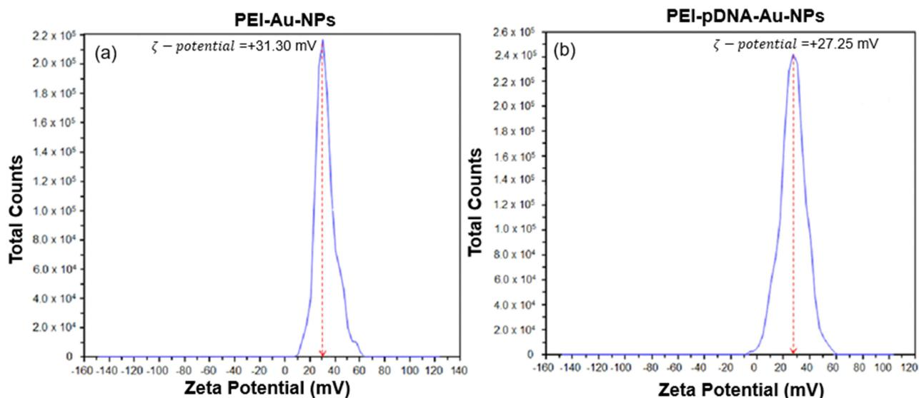
**Figure 6** Zeta-potential values of 4th-generation Au-NPs linked with PEI (a). And PEI-Au-NPs conjugated with plasmid DNA (b). PEI conjugation significantly shifts the zeta potential towards positive values, indicating an increase in the surface charge of Au-NPs. This positively charged surface facilitates electrostatic interaction with the negatively charged cell membrane, promoting cellular uptake of the PEI-Au-NPs and PEI-pDNA-Au-NPs complex.
