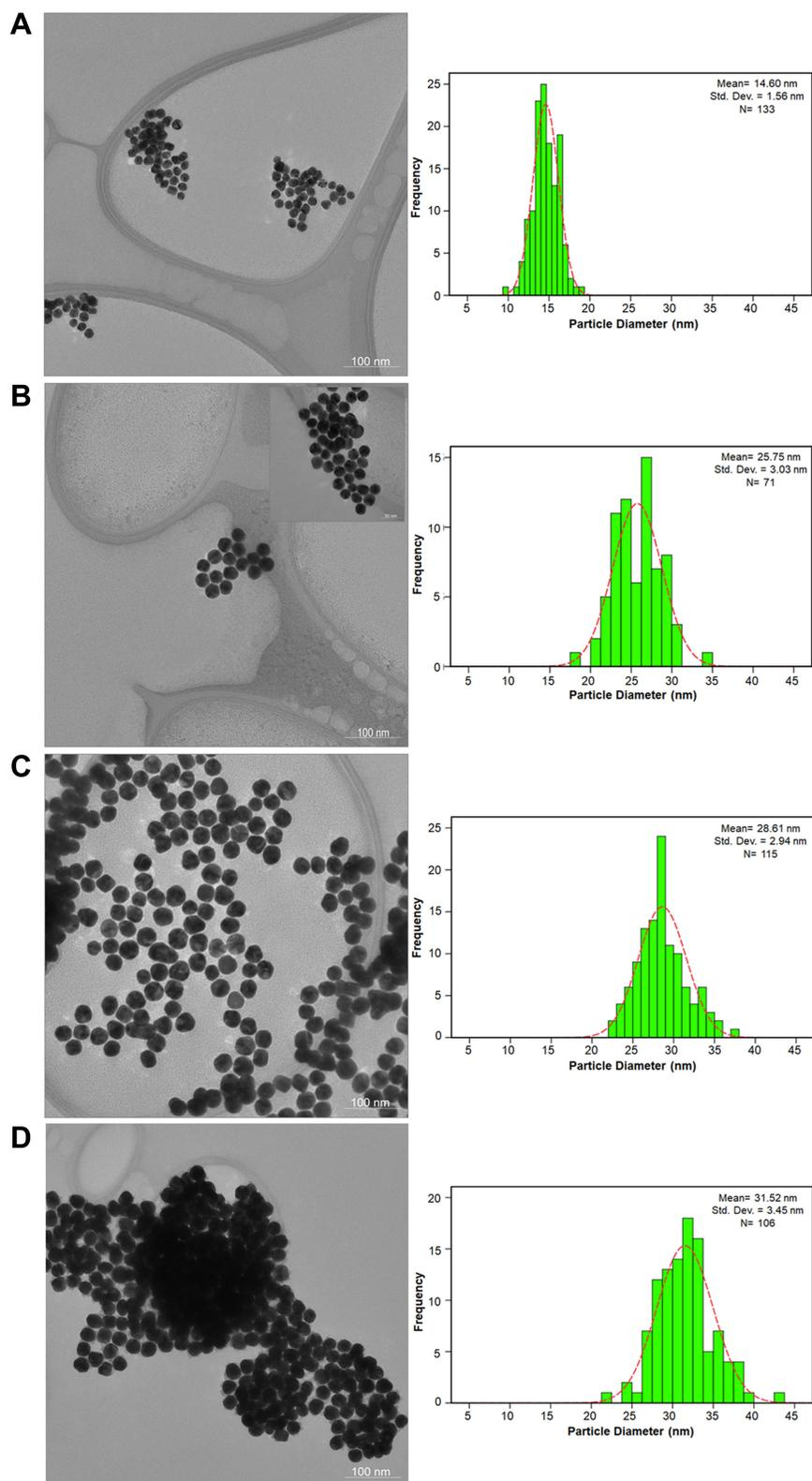
**Figure 4** TEM images and their respective histograms illustrate the sequential stages of Au-NP synthesis via the Turkevich method. These representations capture the four progressive steps (A–D) in the nanoparticle growth process.
