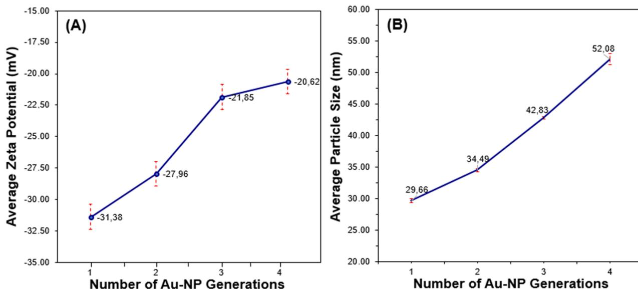
**Figure 5** The images in parts (A and B) demonstrate a reduction in the absolute magnitude of the  $\zeta$  potential concurrent with an increase in Au-NPs size across generations, correlated with alterations in colloidal stability.
