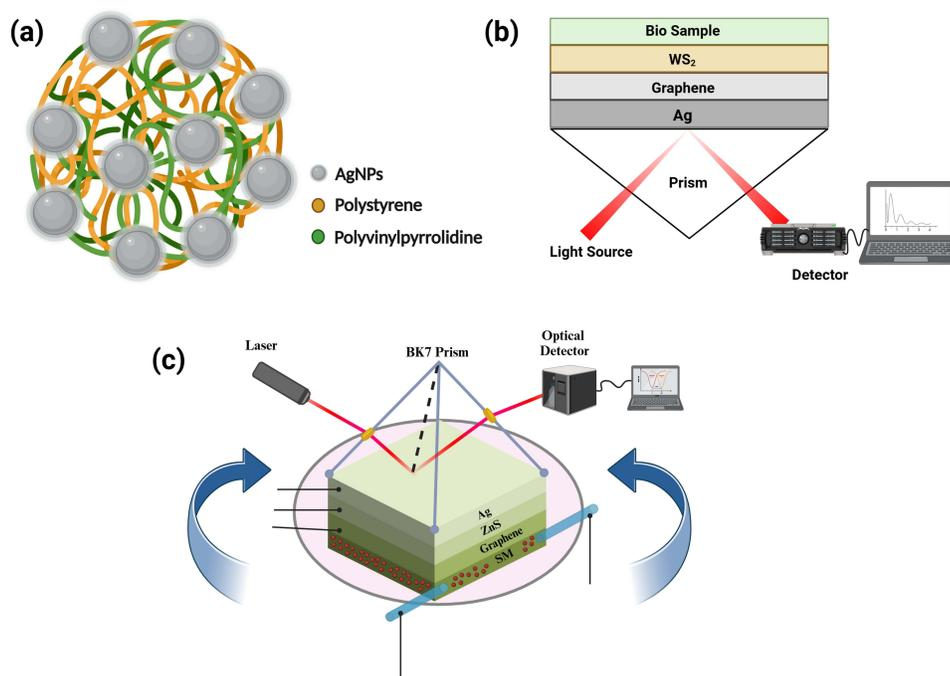
**Figure 3** (a) Schematic illustration of structure and design of a silver nanoparticle (AgNP)-based polymer optical biosensor. (b) Illustration depicting the conceptualized five-layer surface plasmon resonance (SPR) biosensor architecture utilizing graphene-WS<sub>2</sub> for the specific purpose of detecting glucose in urine. (c) Illustration of the configuration of a stratified SPR biosensor.
