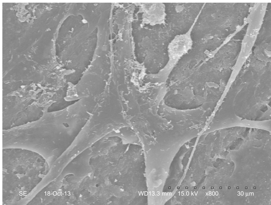
Figure 5 Scanning electron micrograph of mesenchymal stem cells on the surface of the n-HA/PA66/GF composite after 3 days of coculture.
