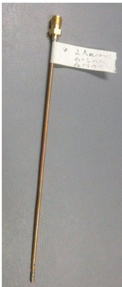
Figure 1 Applicator for microwave ablation.
