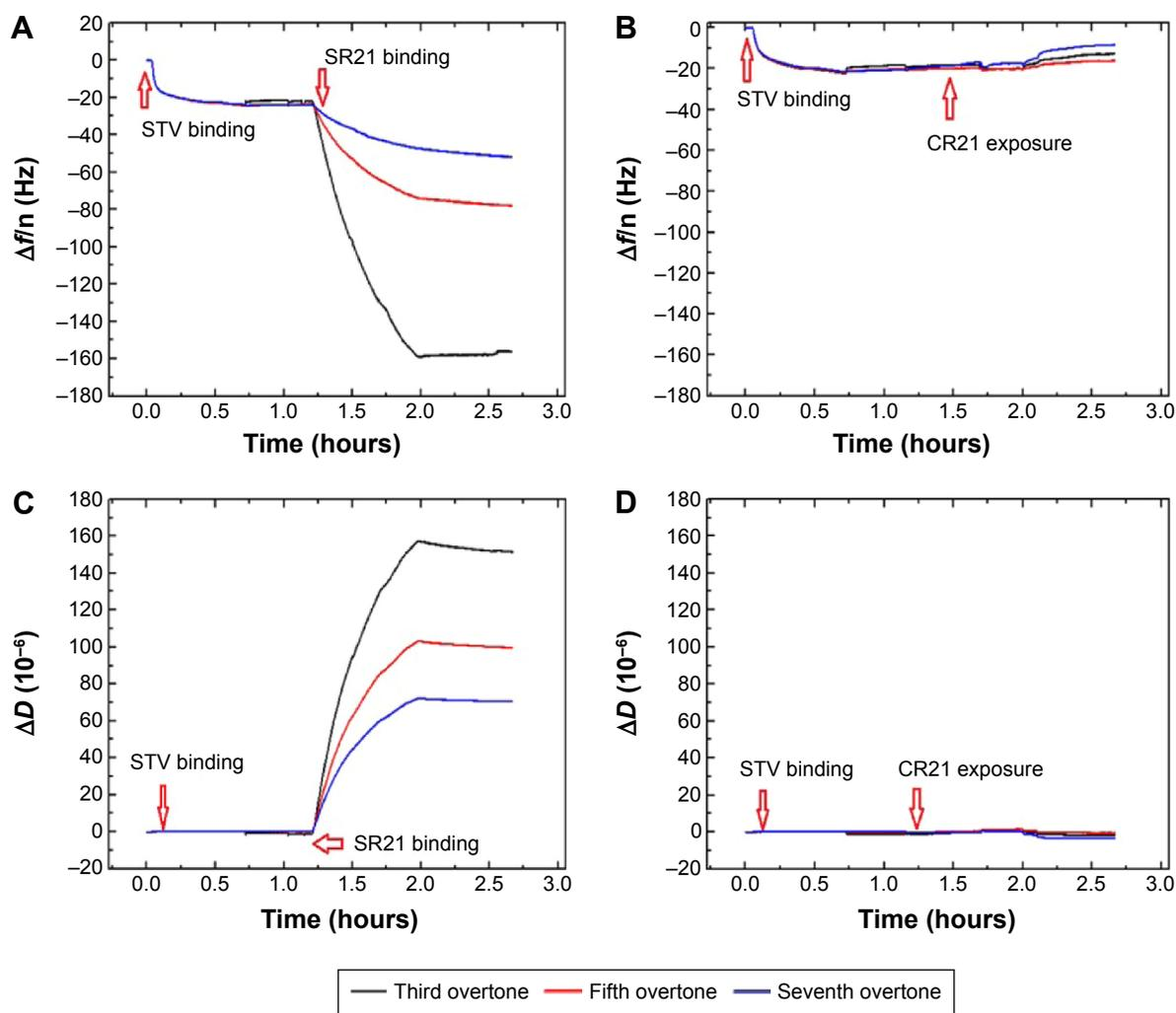
**Figure 1**  $\Delta f$  and  $\Delta D$  responses upon STV adsorption and subsequent binding of SBP displaying phage SR21 (**A** and **C**) and non-SBP displaying CR21 (**B** and **D**) to the Au-coated QCM-D sensors. The red arrows indicate the time of addition of the sample.
