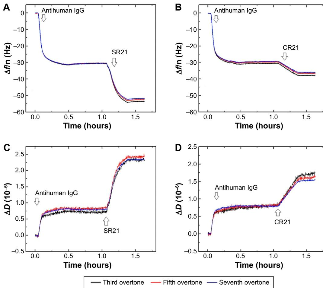
**Figure 5** Characterization of antihuman IgG adsorption and subsequent binding of positive complex (A and C) and negative complex (B and D) to the Au-coated QCM-D sensors. The arrows indicate the time of addition of the sample. **Abbreviation:** QCM-D, quartz crystal microbalance with dissipation monitoring.
