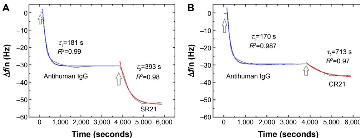
**Figure 7** Kinetic study on adsorption of IgG to Au-coated QCM-D sensors and subsequent binding of positive complex (A) and negative complex (B) for overtone seven. **Notes:** The solid lines represent the fits to Equation 1:  $\Delta f = \Delta f_0 + Ae^{-t/\tau}$ . The arrows indicate the time of addition of the sample. **Abbreviations:** QCM-D, quartz crystal microbalance with dissipation monitoring; A, amplitude;  $\tau$ , time constant.
