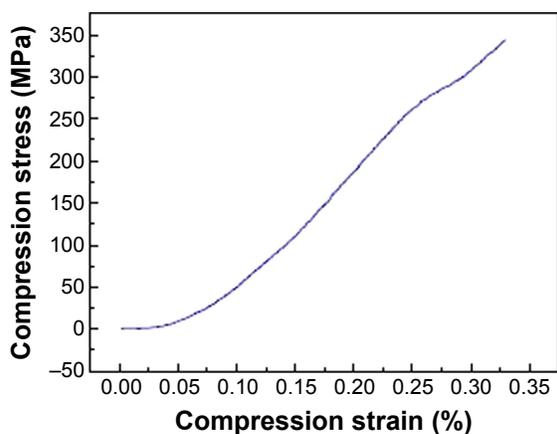
Figure 9 The compression stress–strain curve of wollastonite.
