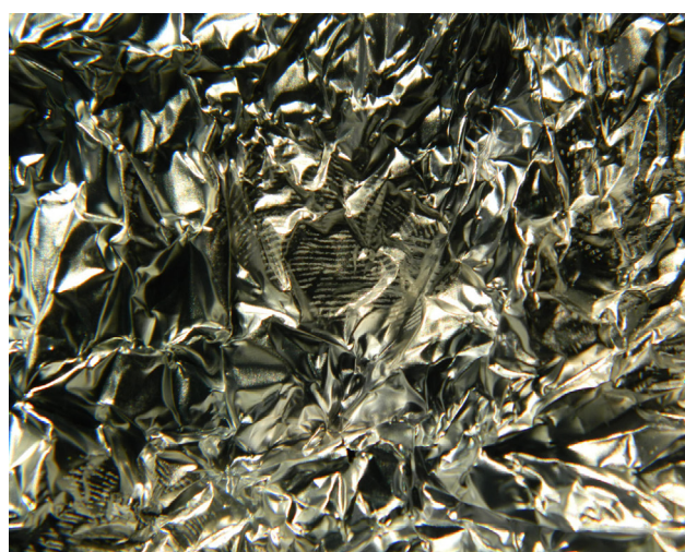
Figure 9 The completely developed latent fingerprint of grade 4 on uncrumpled aluminum foil with the cyanoacrylate fuming.
