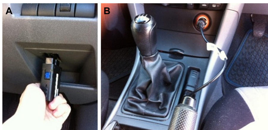
Figure 3 In-vehicle driver monitoring device inserted either into the On Board Diagnostic II (OBD II) port of the vehicle (A) or the cigarette lighter (B).
