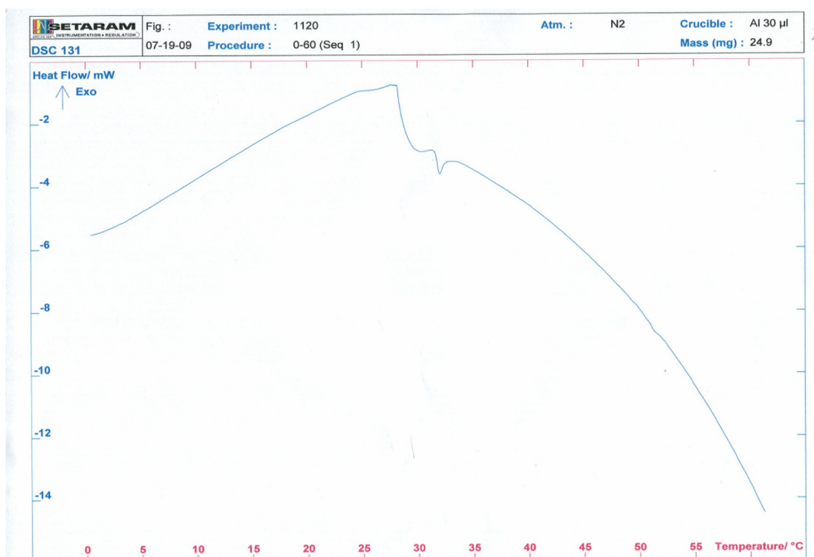
Figure 11 Differential scanning calorimetry spectra of the grafted polystyrene by \gamma -ray (radiation dose: 40 KGy).
