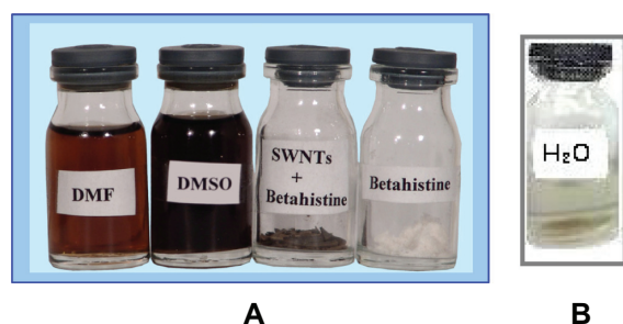
Figure 3 Solubility of grafted SWCNT–betahistine A ) in dimethylformamide (DMF) and dimethylsulfoxide (DMSO) and B ) in \text{H}_2\text{O} .
