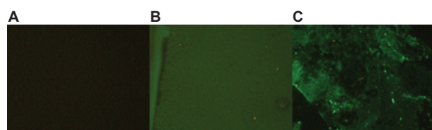
Figure 5 Fluorescence microscopy characterizations of the 6His-tagged green fluorescent proteins (GFP) adsorption, onto the different quartz surfaces. A) PEG-silane onto \text{SiO}_2 B) \text{SiO}_2 C) PEG-silane plus Ni nanoislands.
