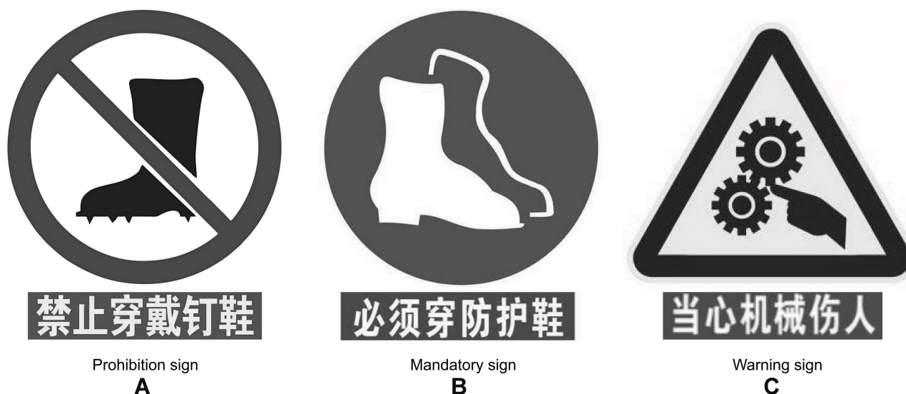
Figure 1 Examples of three types of safety signs: (A) A prohibition sign indicating “No putting on spikes”; (B) A mandatory sign indicating “Must wear protective shoes”; (C) A warning sign indicating “Caution, mechanical injury”.
