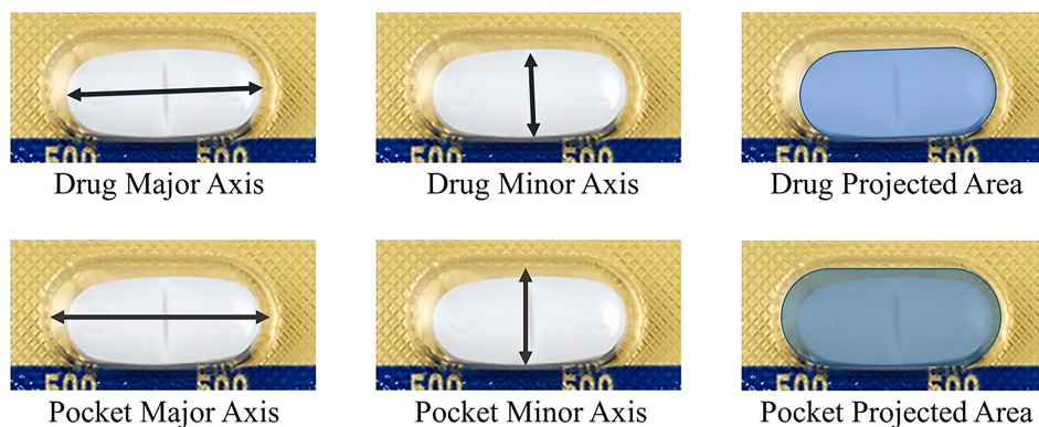
Figure 3 Parameters relating to the inside of PTP pockets.
