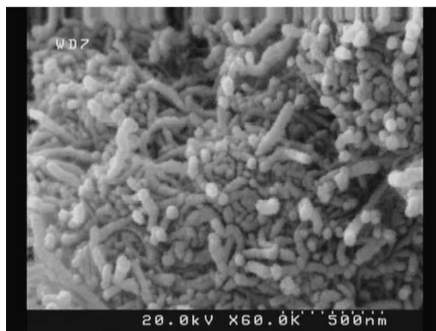
Figure 4 SEM images of MWCNTs functionalized with INH.
