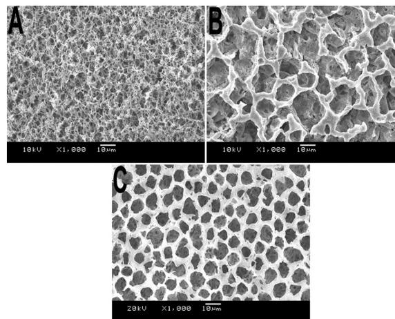
**Figure 4** SEM images of PLA scaffolds prepared with various types of ventilation. **A)** Hermetic environment, **B)** open environment without air, and **C)** open environment with ventilated pumping equipment.
