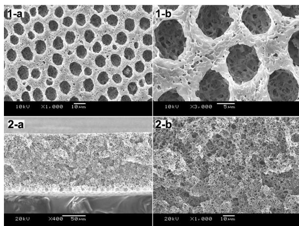
**Figure 5** SEM images of PLA scaffolds prepared at 25°C with the concentration of 10% (w/v). Morphology observation of PLA film included the air face and cross-section: **1-a)** air face of 10% PLA film, 1000×; **1-b)** air surface of 10% PLA film, 3000×; **2-a)** cross-section of 10% PLA film, 400×; **2-b)** cross-section of 10% PLA film, 1000×. **Abbreviations:** PLA, poly(D,L-lactic acid); SEM, scanning electron microscope.
