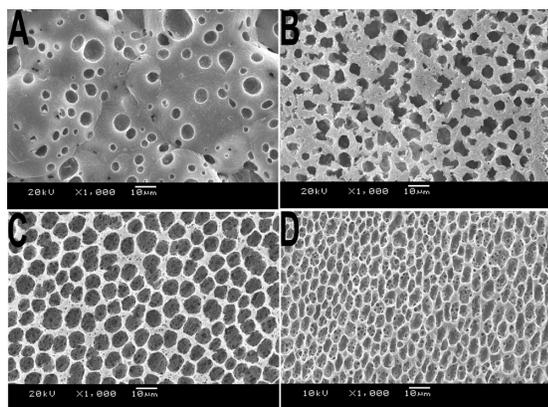
**Figure 2** SEM of morphology of PLA film prepared via different methods. **A)** Volatilization naturally; film prepared via SNS phase separation at the concentration of **B)** 5%, **C)** 10%, and **D)** 15%. All samples were prepared at room temperature without air.
