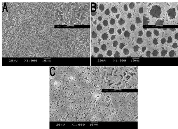
**Figure 3** SEM micrographs of various types of PLA porous scaffold prepared at different temperatures. **A)** 4°C, **B)** 25°C, and **C)** 50°C. Inset: images of corresponding scaffold at higher magnification
