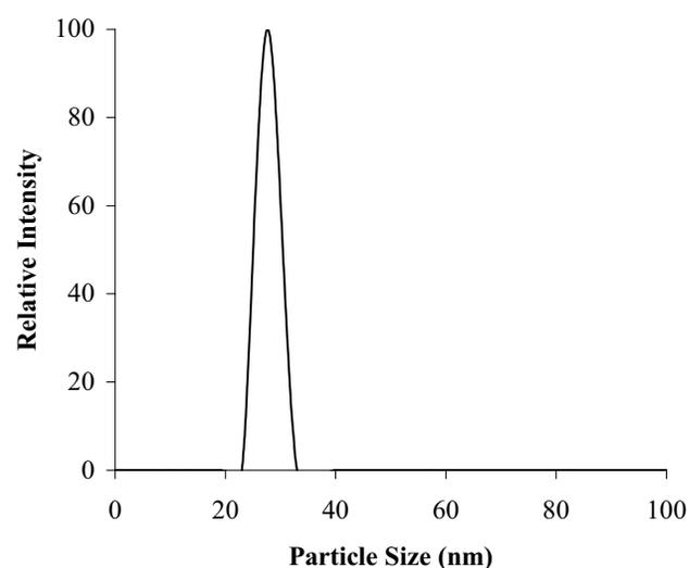
**Figure 1** Dynamic light scattering size-distribution profile for mercaptoacetic acid (MAA)-capped quantum dots (QDs). After sonicator treatment and silica gel separation, particle size distribution was narrowed down to the range between 20 and 35 nm. The mean particle diameter was 27.7 nm.
