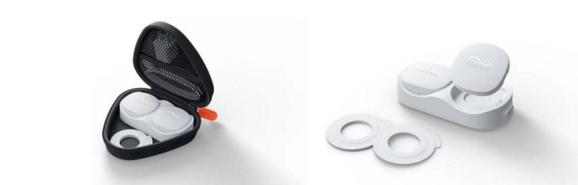
Figure 1 Pictures of the experimental device. Left shows the pods resting in the charging cradle inside the carrying case. Right shows pods, charging cradle, and two adhesive rings.
