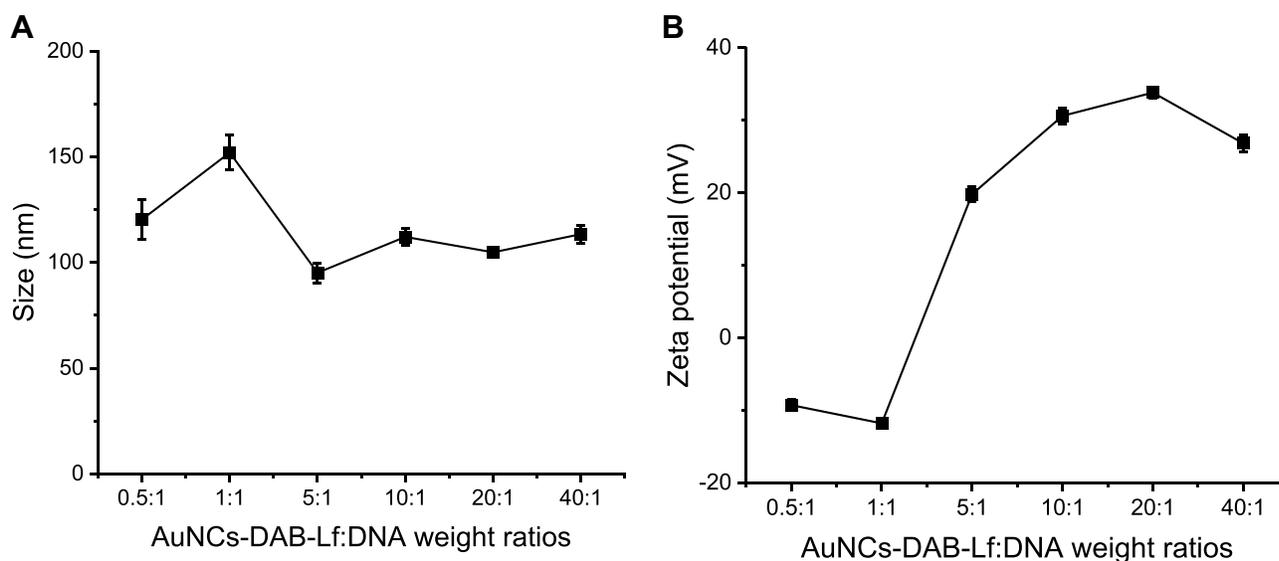
**Figure 3** Size (A) and zeta potential (B) of AuNCs-DAB-Lf complexed with DNA at various AuNCs-DAB-Lf: DNA weight ratios. Results are expressed as mean  $\pm$  SEM ( $n = 9$ ) (error bars smaller than symbols).
