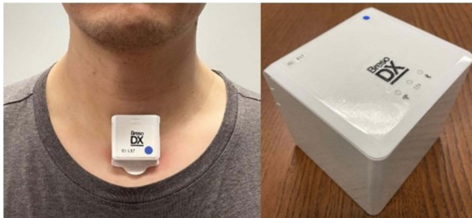
Figure 1 The BresDXI and its computing module, which simultaneously collects trachea-sternal motion and tracheal sound from the BresDXI and SaO 2 from the pulse oximeter.
