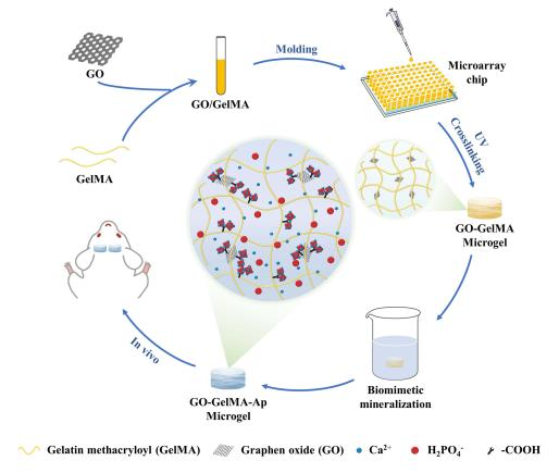
Figure I Schematic diagram of the synthesis of GO-GelMA-Ap microgels and application to cranial bone defect.
