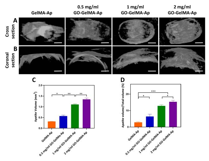
Figure 5 Micro-CT analysis of the microgels. (A) cross-section and (B) coronal section images of microgels. Scale bar = 500  $\mu$ m. (C) Apatite volume (AV) and (D) the apatite volume fraction (AV/TV) of microgels. \* p < 0.05, \*\* p < 0.01, \*\*\* p < 0.01.
