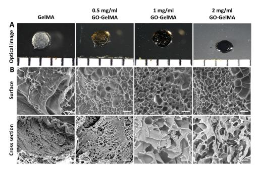
Figure 2 Optical and SEM image of the microgels before biomineralization. (A) Optical image of GelMA, 0.5, I, and 2 mg/mL GO-GelMA microgels; (B) surface and cross section SEM image of the microgels before biomineralization. Scale bar = 20 μm.
