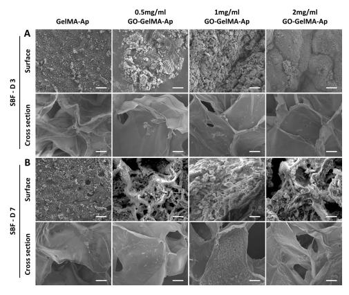
Figure 3 Surface and cross-sectional SEM images of the microgels after biomineralization for 3 and 7 days. Scale bar = 10 µm (A and B).
