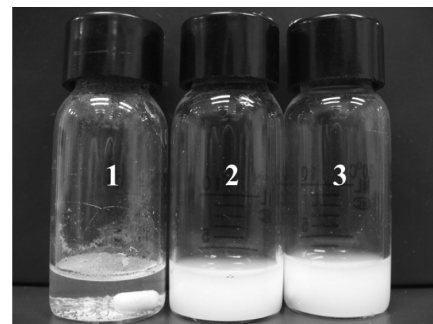
Figure 8 Pyrene (2.47 mM) in water (1) and with R3 (2, 100 \mu\text{M} ), or R4 (3, 100 \mu\text{M} ) in aqueous solution after stirring for 24 hours.
