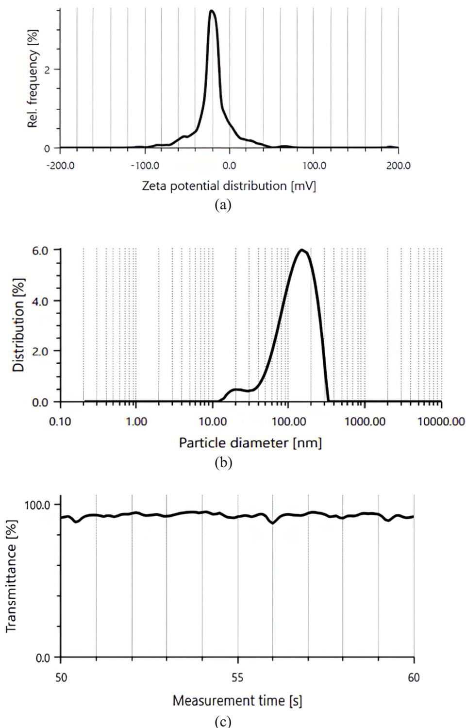
**Figure 6** (a) Zeta potential  $-24.6\text{mV}\pm 0.34$  which confirms the stability of emulsion droplets (b) droplet size,  $129.3\pm 1.57\text{nm}$  showed enhanced total surface area which helped to increase the drug release and (c) % transmittance  $94.82\pm 0.61$  showed confirmation of emulsion in nanometric size of the optimized batch of rhein-loaded liquid nanoemulsion (RL-SNEDDS) (F7).
