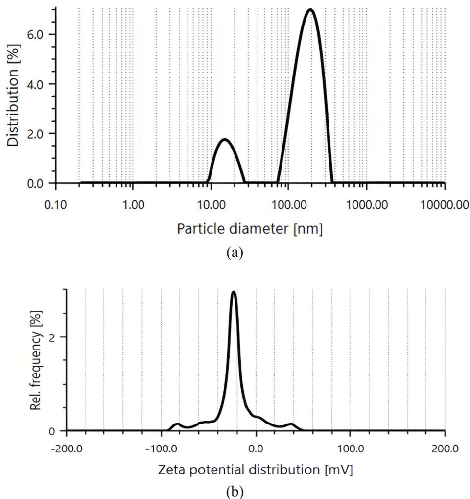
**Figure 7** (a) Particle size of rhein-loaded solid nanoemulsion (RS-SNEDDS) was  $142.3 \pm 1.67 \text{ nm}$  with polydispersity index  $0.21 \pm 0.001$  confirming the nanoparticle size and uniformity of particles after solidification and (b) zeta potential  $-23.4 \pm 1.06 \text{ mV}$  confirming the nanocarrier stability.
