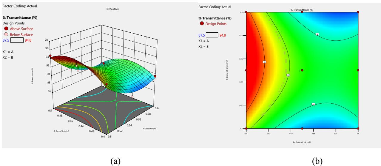
**Figure 3** (a) 3D response graph and (b) contour plot for the effect of concentration of eucalyptus oil and surfactant: cosurfactant ( $S_{mix}$ ) on % transmittance shows that as  $S_{mix}$  concentration raised, the % transmittance also increased and decreased with eucalyptus oil concentration increased.
