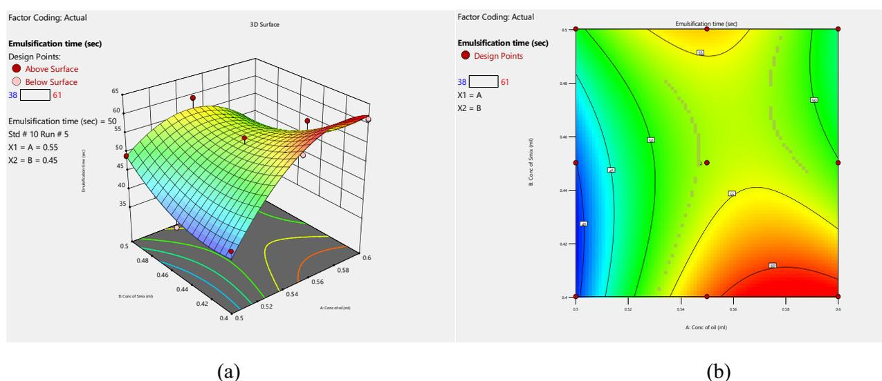
**Figure 4** (a) 3D response graph and (b) contour plot for the effect of concentration of eucalyptus oil and surfactant: cosurfactant ( $S_{mix}$ ) on emulsification time shows that the emulsification time decreased with the increased concentration of  $S_{mix}$  and the emulsification time increased with increased oil concentration.
