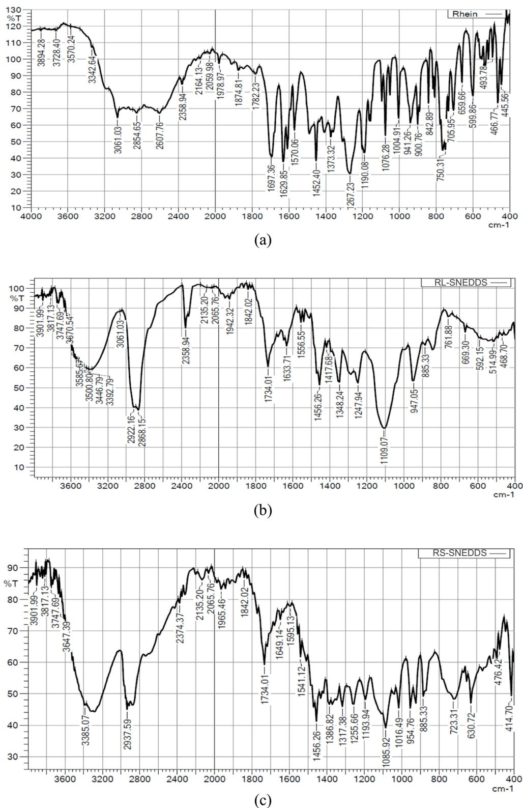
**Figure 8** Fourier Transform Infrared Spectroscopy of (a) rhein, (b) rhein-loaded liquid nanoemulsion (RL-SNEDDS), and (c) rhein-loaded solid nanoemulsion (RS-SNEDDS) confirm the hydrophobic interaction of rhein with eucalyptus oil and PEG-400 forms a complex with eucalyptus oil and  $S_{mix}$  after its entrapment and helps to enhance solubilization.
