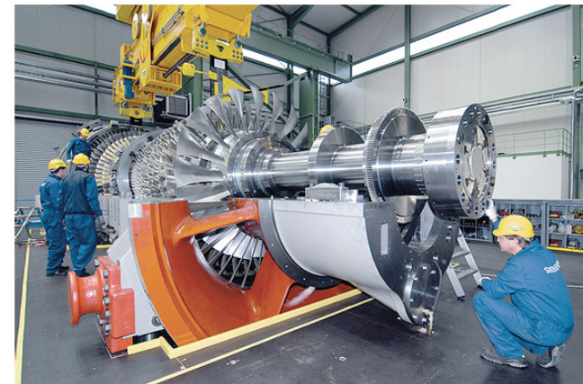
Siemens SGT5-8000H 375MW Gas Turbine
